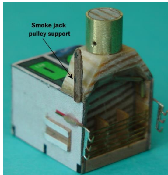
Figure N88 - Smoke jack pulley support fitted
