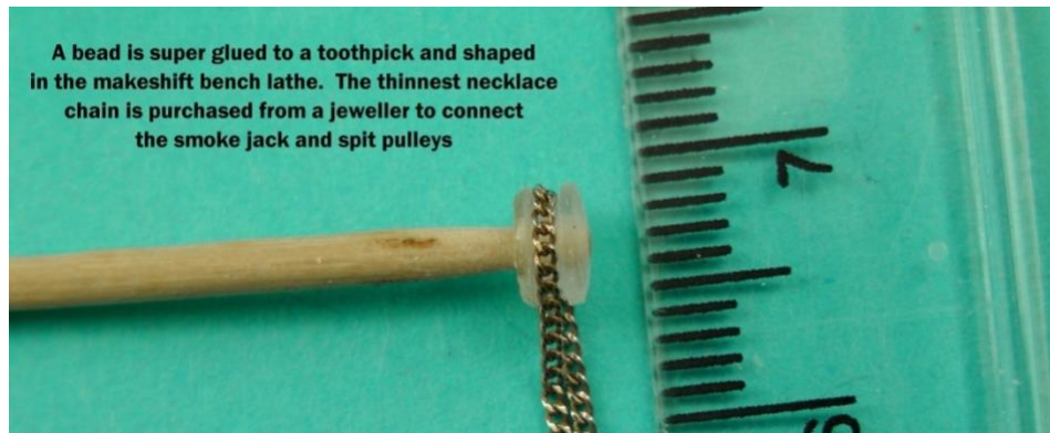
Figure N79 - Spit pulley shaped to fit necklace chain
