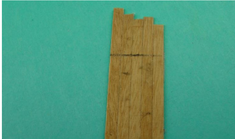
Figure N25 - Square edge drawn on the planks
