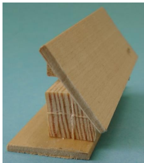
Figure N101 - Support for back rail whilst it is being soldered to the side rails
