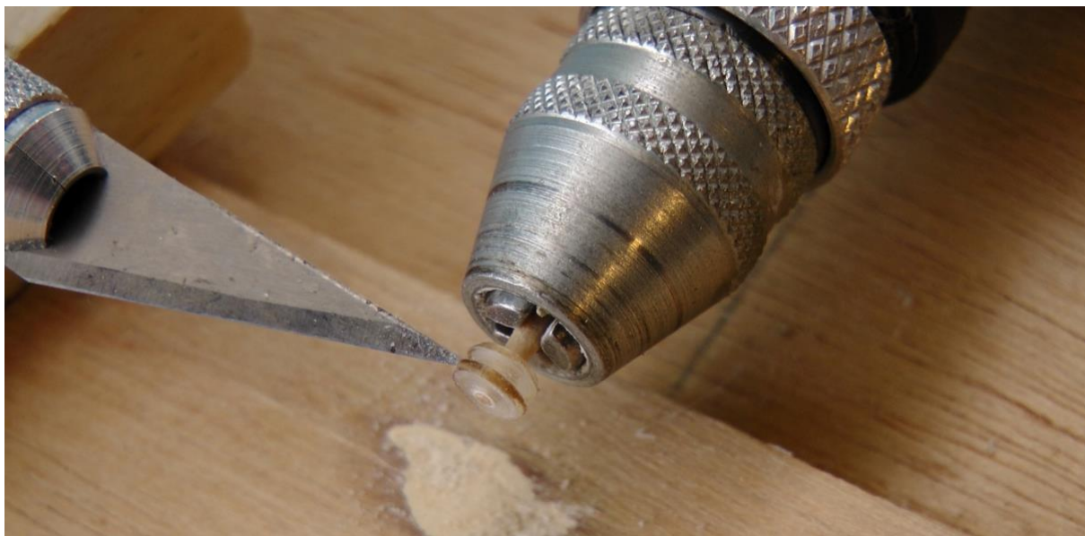
Figure N78 - Craft drill adapted as a bench lathe to shape the pulleys
