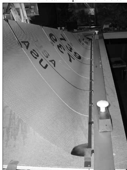
Photo 2: Main luff measurement.
