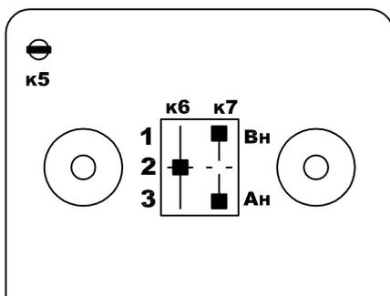
Model is submerged and in neutral buoyancy (K5 and K6 centered):
