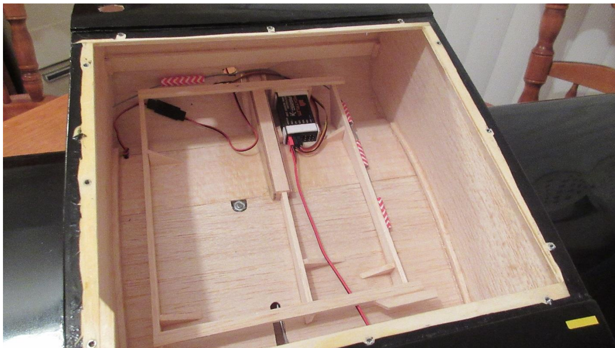
The receiver is tucked discretely under the fuel tank platform.
