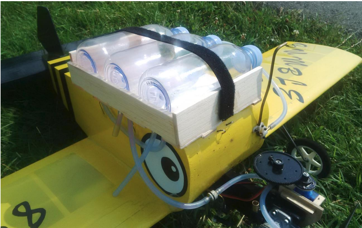
Design testing of horizontal cylinders plumbed in various ways.
