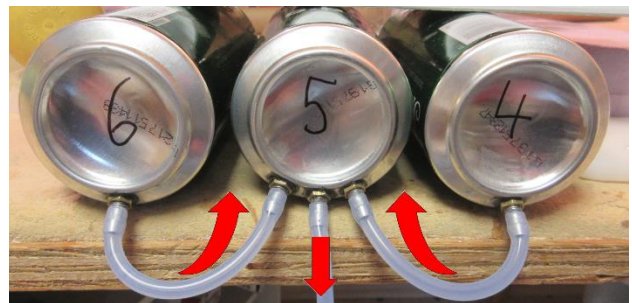
Parallel plumbing provides a smooth fuel level drop of all three tanks simultaneously.
