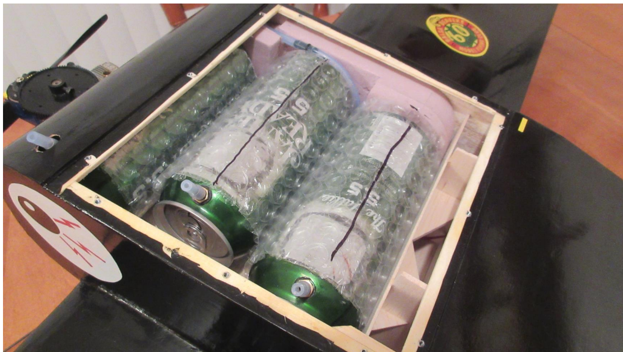
Bubble wrap makes excellent lightweight packing. No extra weight is carried in endurance, so a "snug fit" is used to hold the tanks in place rather than heavy straps and mounts.
