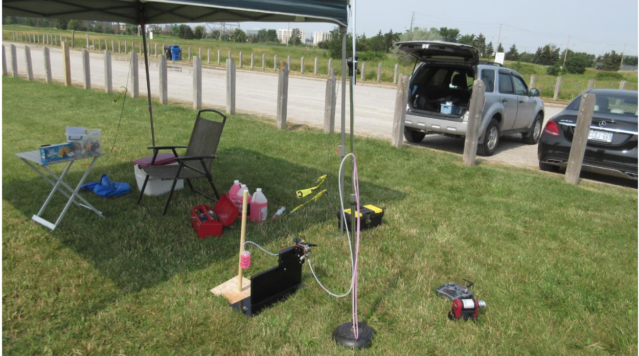
A home-made manometer measuring muffler pressure.
