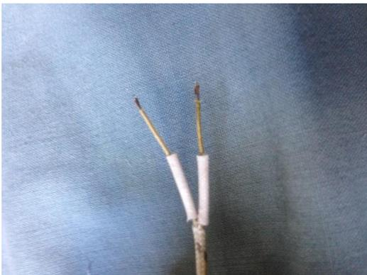
The white supplied cable will need to be striped back about 20mm and the both inner cables will need to also be striped to 5mm.
