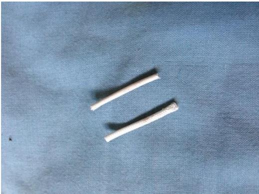
Once the cables have been unsoldered and removed the white insulators can be taken off.
