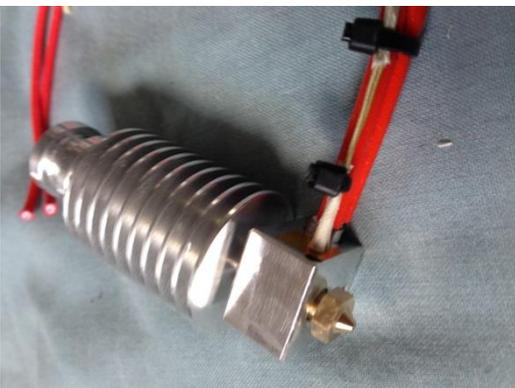
Screw the heat sink on.
