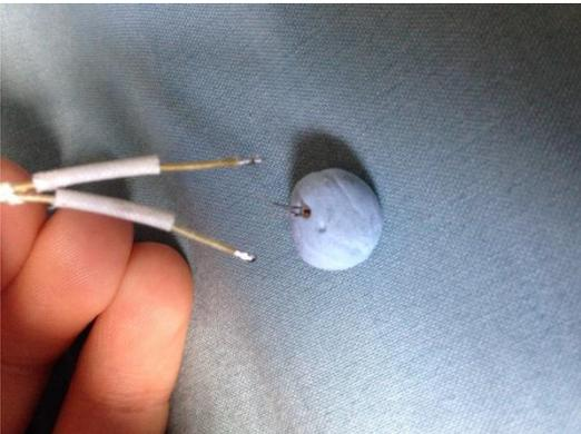
Solder both the wires to the two thermistor legs.
