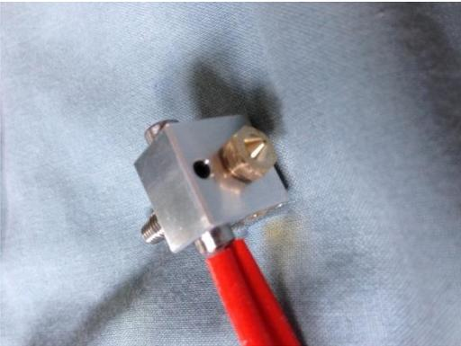
Secure the heater cartridge into the heat block with the grub screw.
