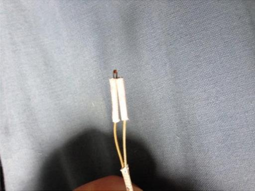
Slide the two insulating sleeves up to the thermistor.
