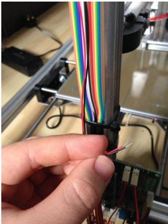
Run the cables along the route of the cable tape towards the control board.
