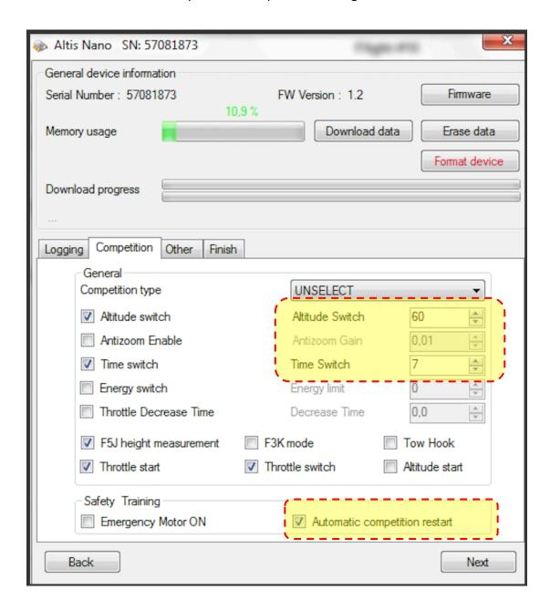
In this menu you have to program the Nominal Launch Height. In this example the Altitude Switch is 60 meter and the Time Switch is set on 7 seconds. Also select "Automatic Competition restart". With these settings, the Altis is automatically reset in case the height is below 8 mtr. This setting is important as we fly multiple start during one F5K task.
