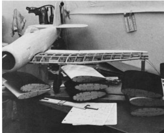
Airfoil, test sections actually used to prepare graphs.
